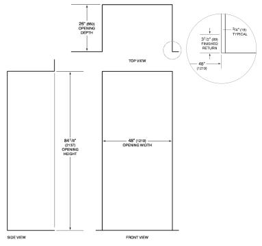
NOTE:  $3^{7}/2^{\circ}$  (89) finished returns will be visible and should be finished to match cabinetry.
