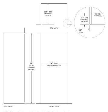
NOTE:  $3^{1}/2^{\circ}$  (89) finished returns will be visible and should be finished to match cabinetry. Requires extra 40mm depth for power socket and water connection.
