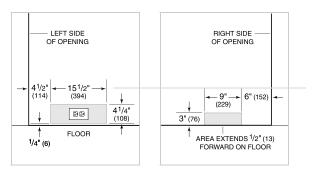
**NOTE:** The electrical outlet must be positioned with the grounding prong to the right of the thinner blades.
