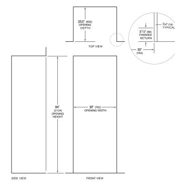
NOTE:  $3^{1/2^*}$  (89) finished returns will be visible and should be finished to match cabinetry. Requires extra 40mm depth for power socket and water connection.
