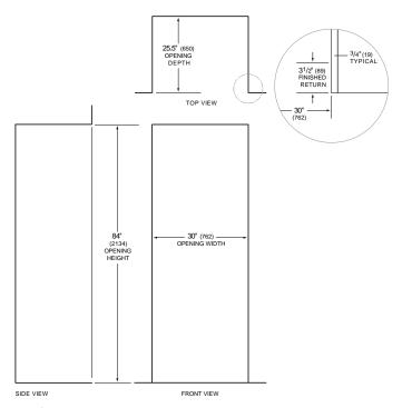
NOTE: 3<sup>1</sup>/2\* (89) finished returns will be visible and should be finished to match cabinetry. Requires extra 40mm depth for power socket and water connection.
