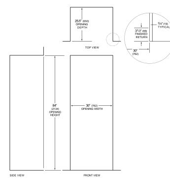
NOTE: 3<sup>1</sup>/2\* (89) finished returns will be visible and should be finished to match cabinetry. Requires extra 40mm depth for power socket and water connection.
