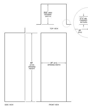
NOTE: 3<sup>1</sup>/2" (89) finished returns will be visible and should be finished to match cabinetry. Requires extra 40mm depth for power socket and water connection.
