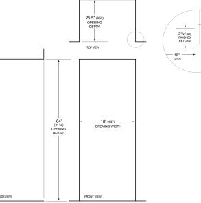
NOTE: 3<sup>1</sup>/2<sup>+</sup> (89) finished returns will be visible and should be finished to match cabinetry. Requires extra 40mm depth for power socket and water connection.
