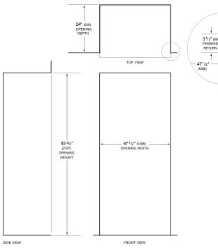
NOTE:  $3^1/2^n$  (89) finished returns will be visible and should be finished to match cabinetry Shaded line represents profile of unit.
