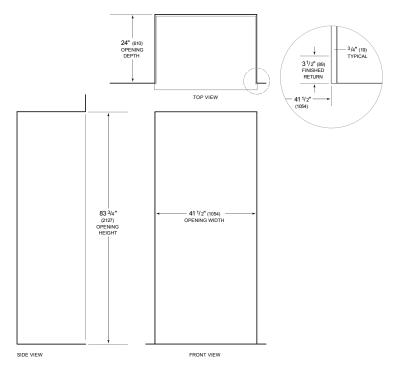
NOTE: 31/2\* (89) finished returns will be visible and should be finished to match cabinetry. Shaded line represents profile of unit. Requires extra 40mm depth for power socket and water connection.
