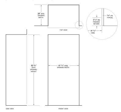
NOTE:  $3^1/2^*$  (89) finished returns will be visible and should be finished to match cabinetry. Shaded line represents profile of unit. Requires extra 40mm depth for power socket and water connection.
