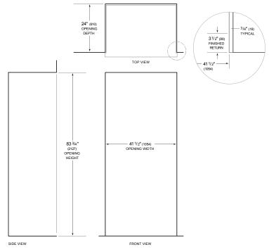
NOTE: 3<sup>1</sup>/<sub>2</sub>\* (89) finished returns will be visible and should be finished to match cabinetry. Shaded line represents profile of unit. Requires extra 40mm depth for power socket and water connection.
