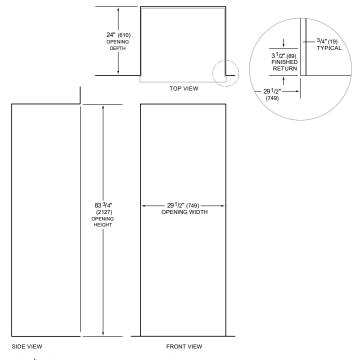
NOTE:  $3^{1/2^{\circ}}$  (89) finished returns will be visible and should be finished to match cabinetry Shaded line represents profile of unit.
