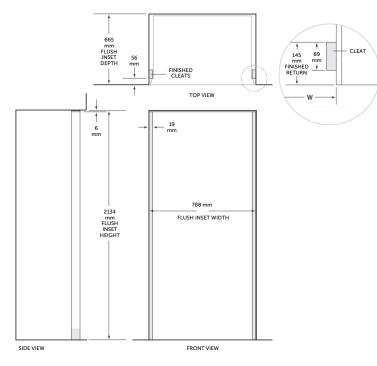
NOTE: 31/2\* (89) finished returns and shaded areas will be visible and should be finished to match cabinetry Shaded line represents profile of unit with\* (19) panel.
