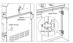
Remove rear bracket and plug. Remove cart door.
