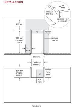
NOTE: Shaded area above countertop indicates minimum clearance to combustible surfaces, combustible materials cannot be located within this area. An insulating liner is not required.
