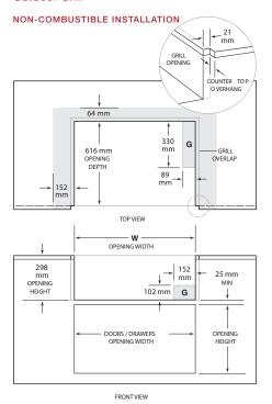
NOTE: Shaded area above counterton indicates minimum clearance to combustible surfaces, combustible materials cannot be located within this area.
