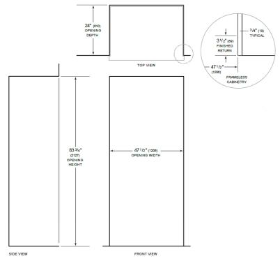
NOTE:  $3^{1}/2^{n}$  (e)) finished returns will be visible and should be finished to match cabinetry Shaded line represents profile of unit.
